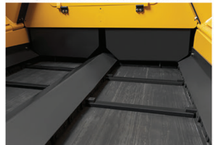
Flow gates, hydraulically controlled
