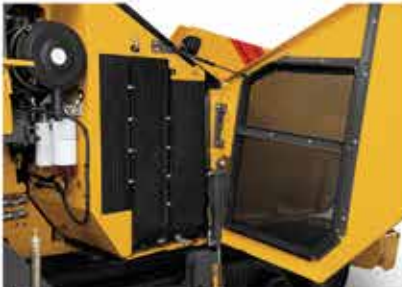
Radiator debris screen
